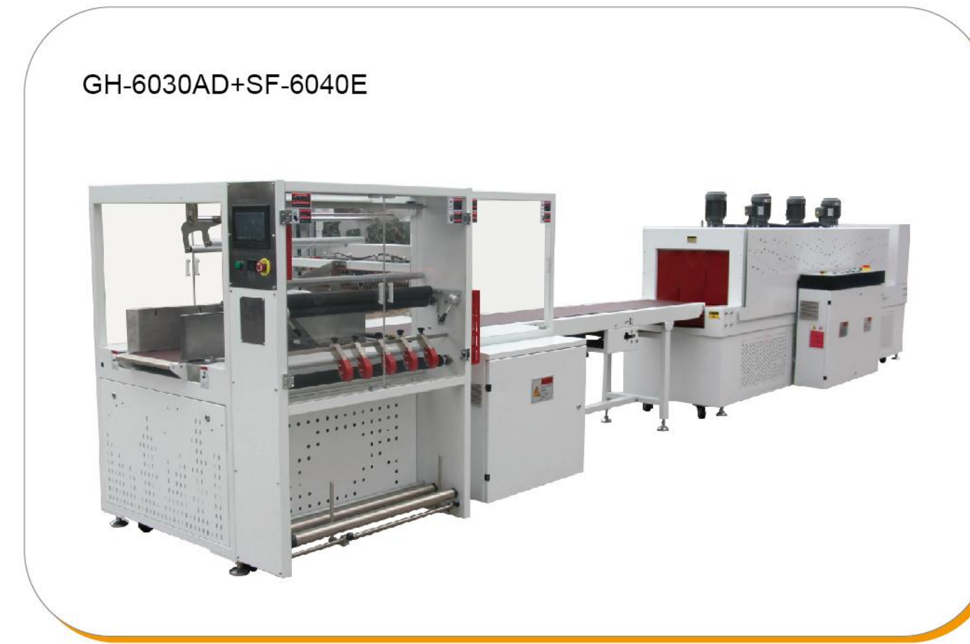
全封闭（对折膜叠膜式）自动封切收缩包装机 Fully-auto Sealing Machine & Shrink Tunnel (Center-folded Film)
